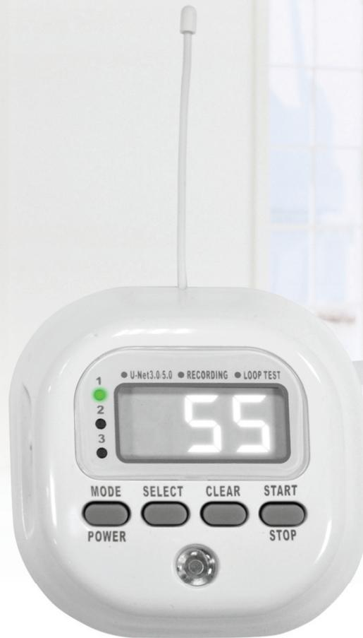
The SQ201 is a simple tool to assist the Installer when trouble shooting RF signal in the customer premise. The device measures RF level on the frequency band used by VIAS devices only. This covers frequency bands for Unet 5.0 and older Unet 3.0 devices.
