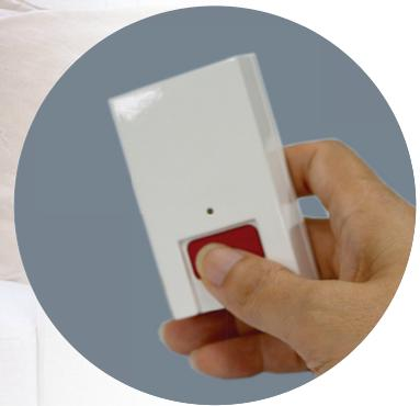
The SR203 is a wireless panic button to allow the user to press for help in emergency situations. When transmitting alarm signals, the SR203 flashes its LED and produces a vibration as confirmation that a panic signal message has been sent to the gateway.
